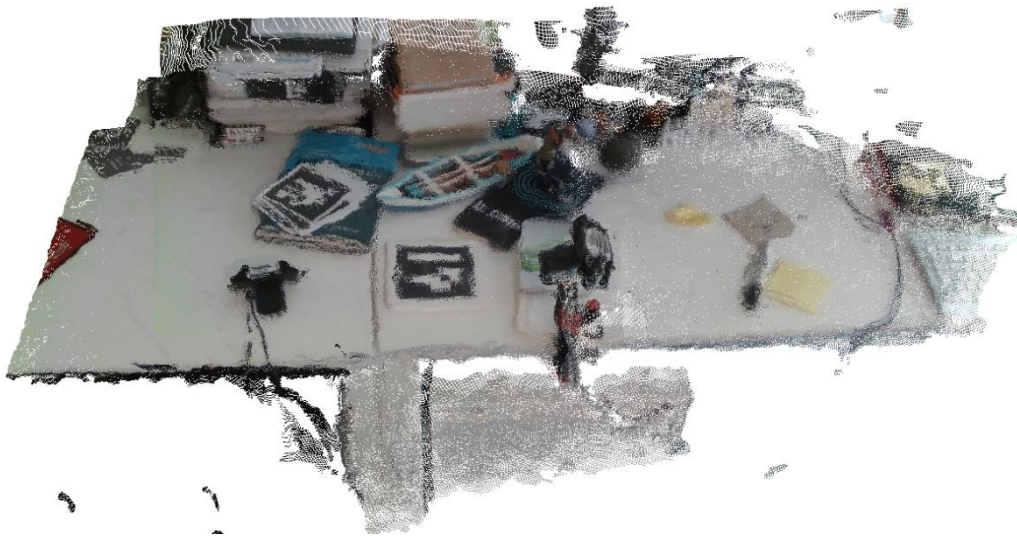
Figure 4-10. A 3D non-feature point cloud is constructed by RealSense camera.
